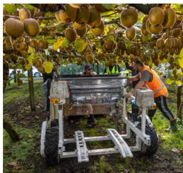
The e-BIN prototype human-assist harvester developed by the University of Waikato.
