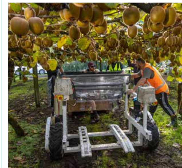
The e-BIN prototype human-assist harvester developed by the University of Waikato.
